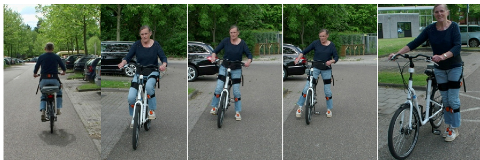
Fig. 2. Getting used to mounting the SOFIE bicycle: stepping through frame, sit on saddle, put one foot on pedal and cycle off while saddle height is increasing.
