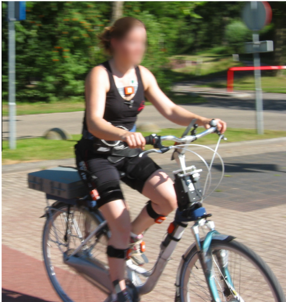
Fig. 1. Attachment of the sensors on the test bicycle and cyclist.
